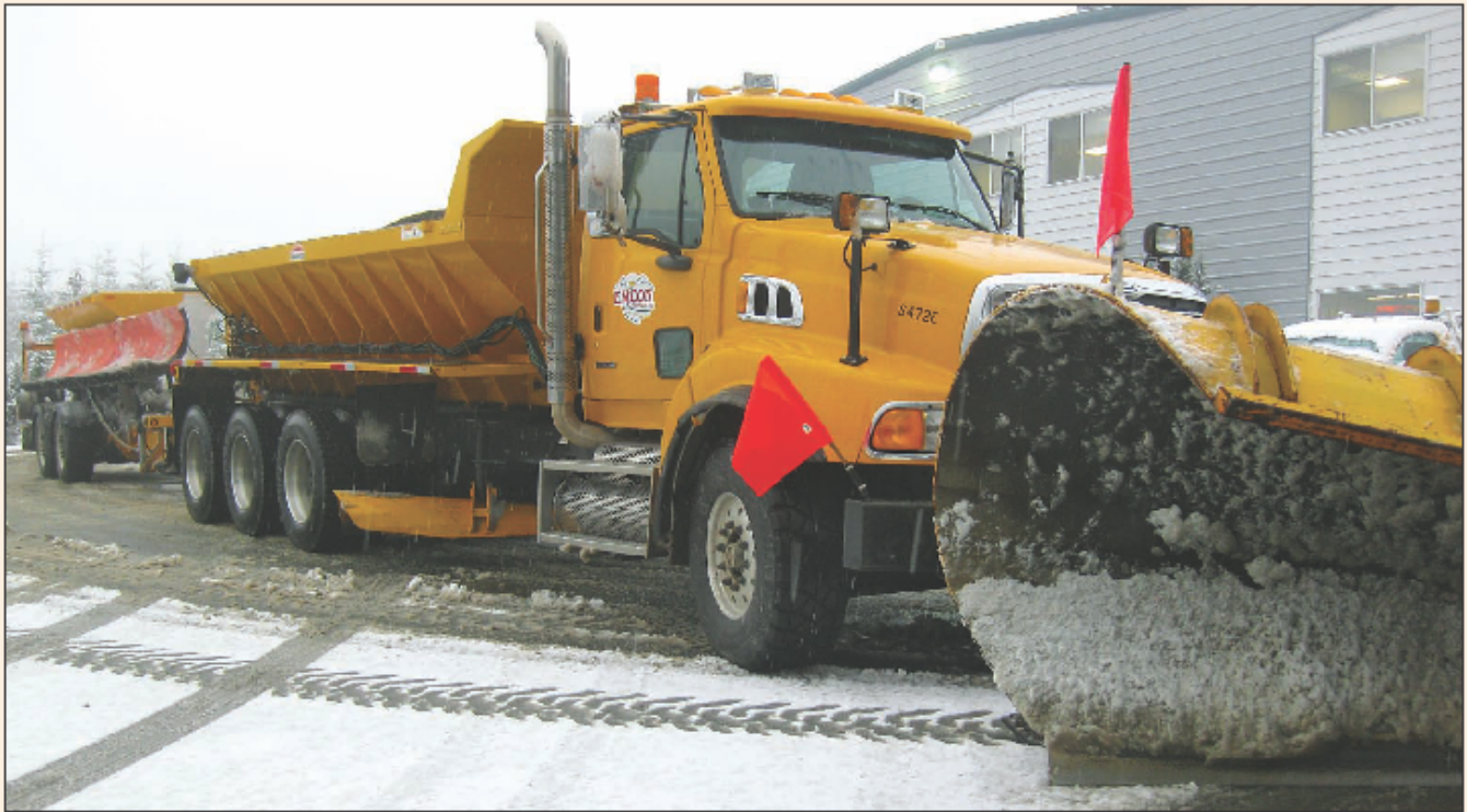
THE IMPRESSIVE-LOOKING Tow Plow is 24 feet wide and 80 feet long and deans roads in a hurry. The Valley has the island's only Tow Plow.
